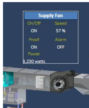
13 Figure 10: VFD points in Equipment Graphic
