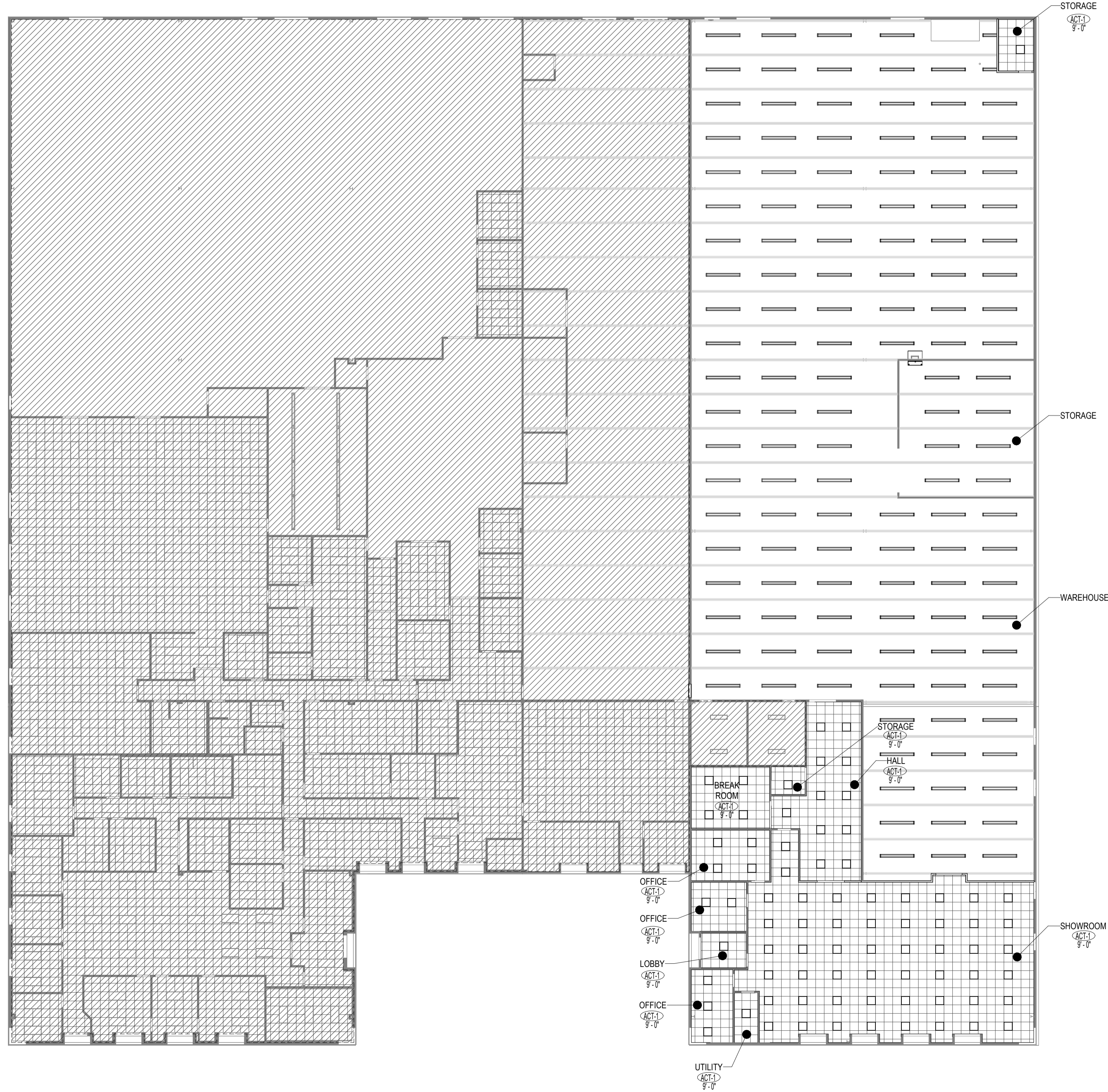
1 REFLECTED CEILING PLAN 1/16" = 1'-0"
